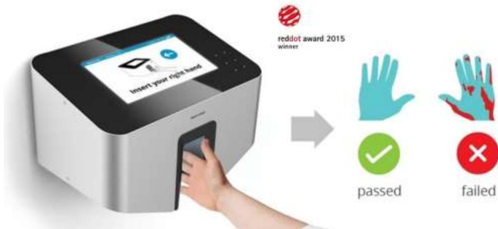
The hand hygiene system, named Semmelweis Scanner, enables immediate evaluation of hand hygiene by detecting the distribution of a special handrub. The objectivity – which is critical in the fight against HAI – is accomplished by the software evaluation of recorded images. The system was validated on over 17,000 healthcare workers and used in 17 countries.
